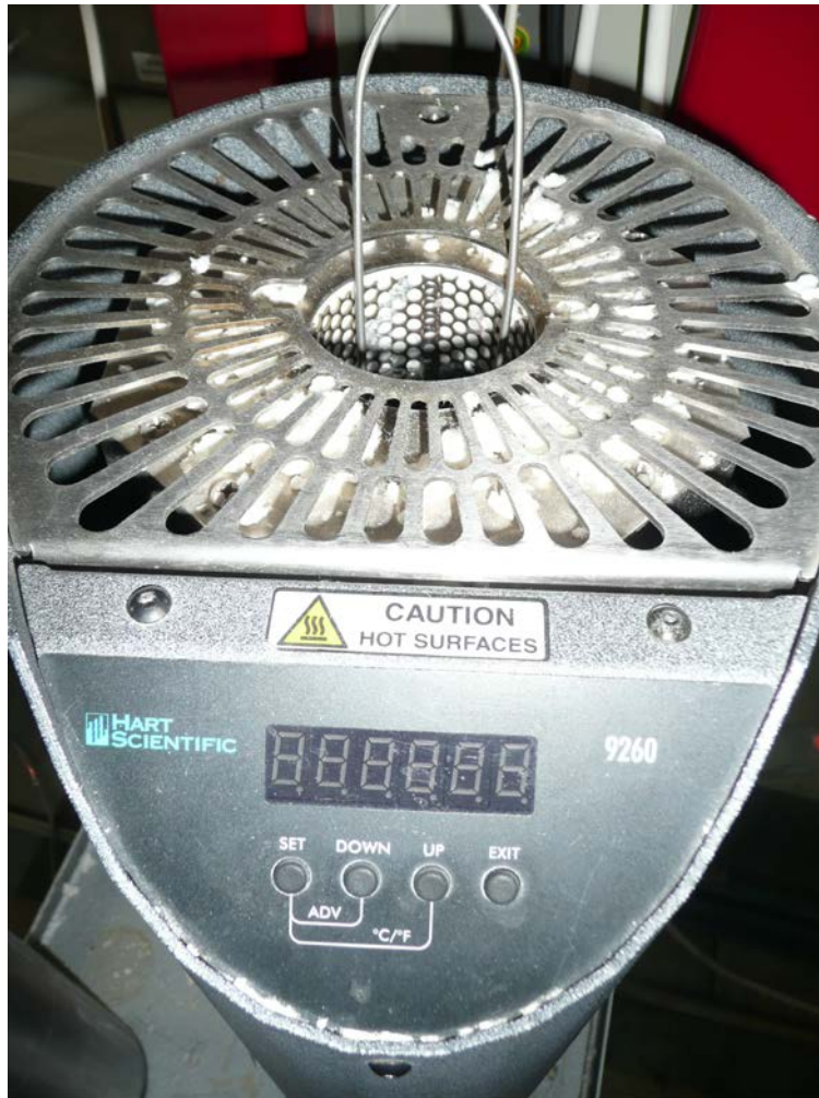
Figure 1. Thermostat Hart Scientific; type: 9260.
