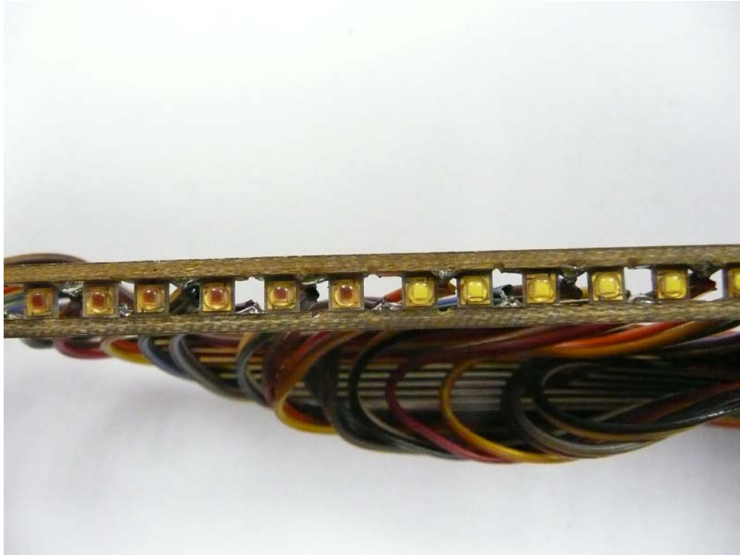
Figure 8. Cabling for the red and white LEDs of PARATHOM CLASSIC A 80 .
