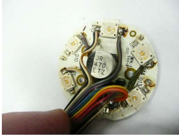
Figure 5. Cabling for Osram Parathom Classic A40.
