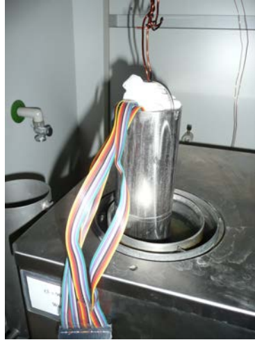
Figure 3. Huber oil bath thermostat. The upper part of the metal tube was well isolated in order to decrease the nonuniformity of the space where the LEDs were located.
