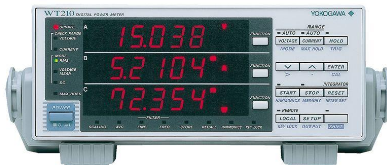
Figure 3. Yokogawa power meter traceable to EL reference standards.
